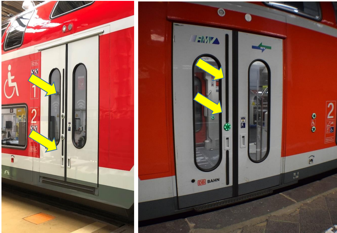
Figure 6.1.1 a-b: View of a train door with tactile aid (blind strip)
