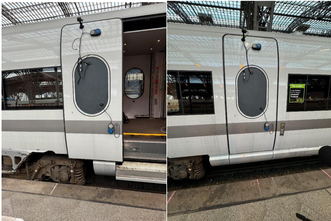
Figure 5.6 a-b: View of the prepared test door (a. open, b. closed)
