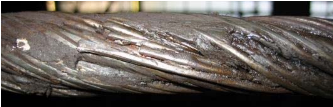
Illustration 11: câble sale - inspection impossible
