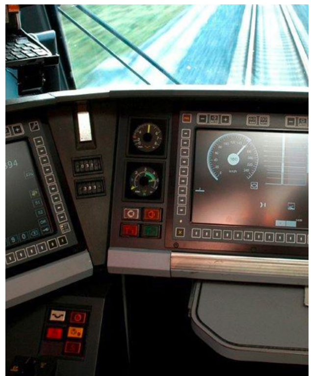
ETCS L2 provides locomotive drivers with information on a screen.
