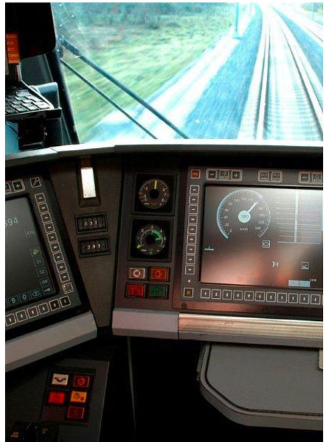
ETCS L2 provides locomotive drivers with information on a screen.
