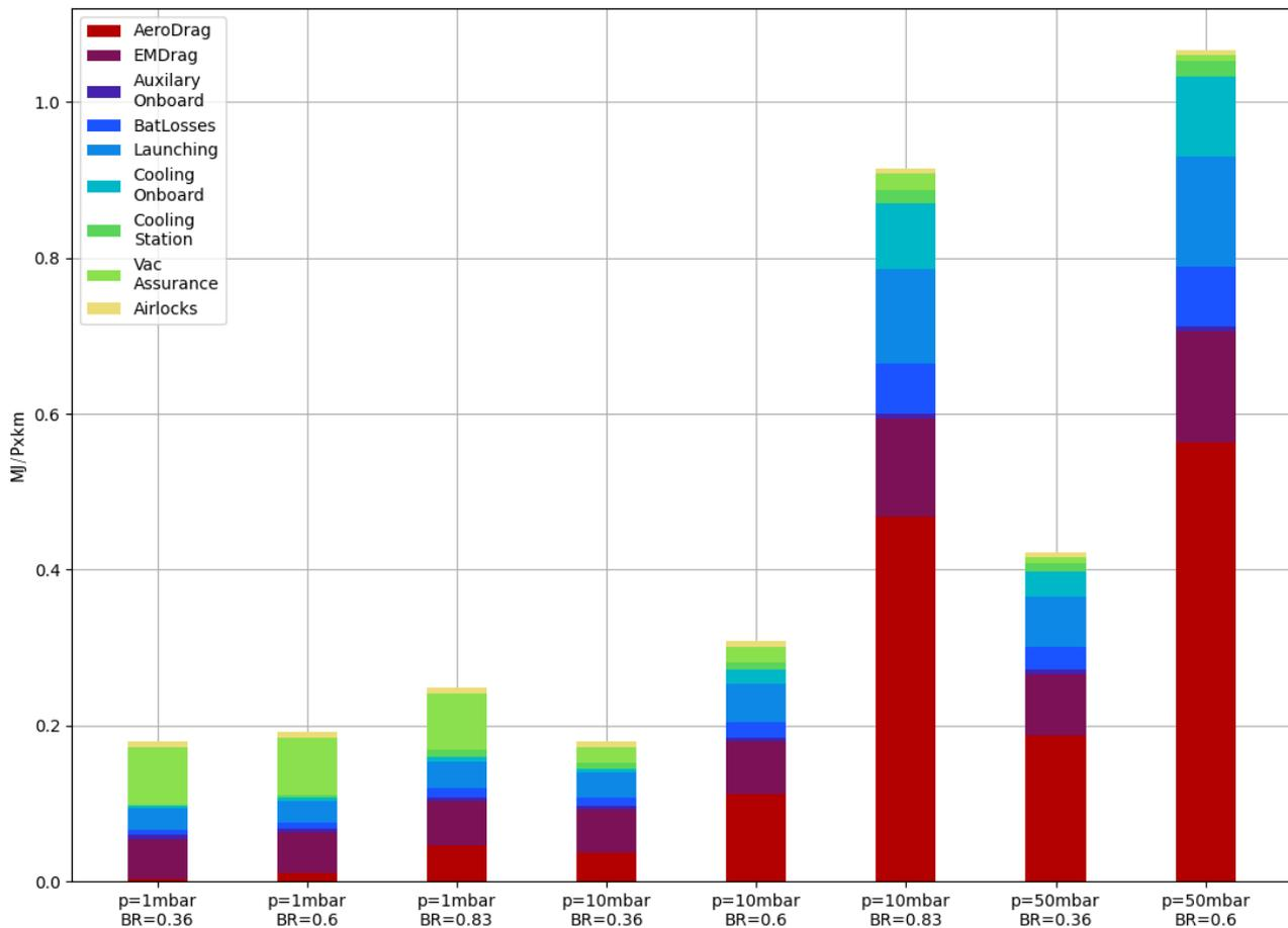
**Fig. 4.1.** Operational energy breakdown for different combinations of blockage ratios (BR) and tube air pressure (p). The combination with p=10 mbar and BR=0.6 corresponds to the reference case.
