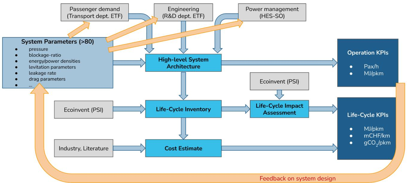
**Fig. 3.1.** Schematic representation of the methodology employed to size the hyperloop system and estimate its KPIs.
