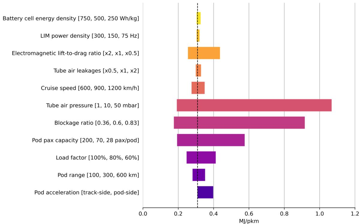
**Fig. 4.2.** Specific energy consumption of the hyperloop system (in MJ/pkm) for various input design settings. Each row explores a different dimension: first and third values correspond to the left and right margins of the bars; the second value is captured by the dashed line and indicates the reference case.
