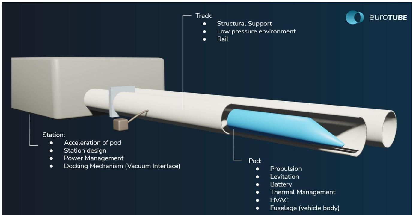
**Fig. 2.1.** Main subsystems of a hyperloop system with the corresponding components
