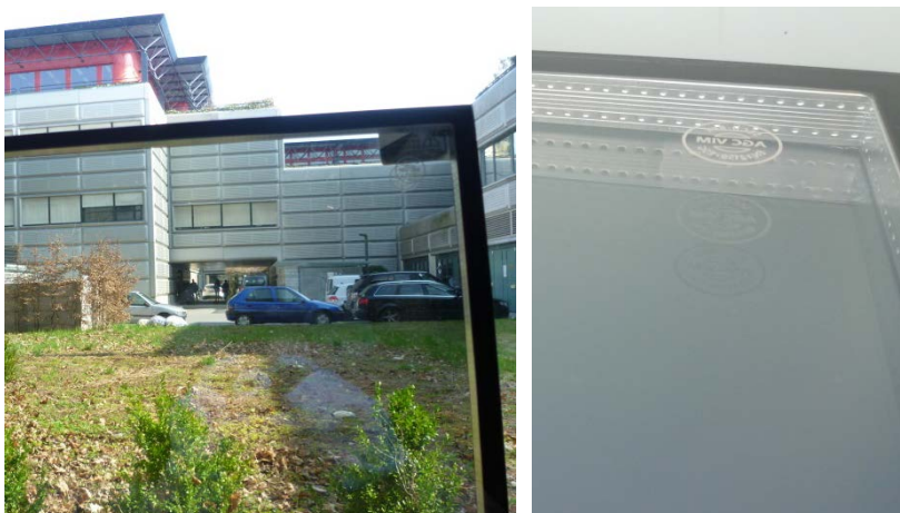
Figure 4 : Photographs of a double glazing with laser structured low-e coating, on the right with light at low incidence angle. The scribed lines are barely visible to the eye
